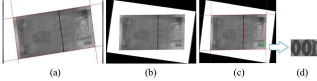
Fig. 2. (a) RMB edge detection, (b) skew correction, (c) RMB security thread, and (d) '100' template
